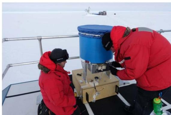
IceACT (Ice Air Cherenkov Telescope) is a compact imaging air-Cherenkov telescope. It is under consideration as part of IceCube-Gen2.
